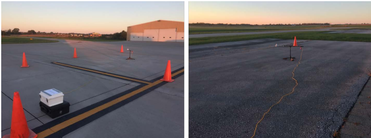
Figure 3.3 Albedo measurement system with an albedometer
